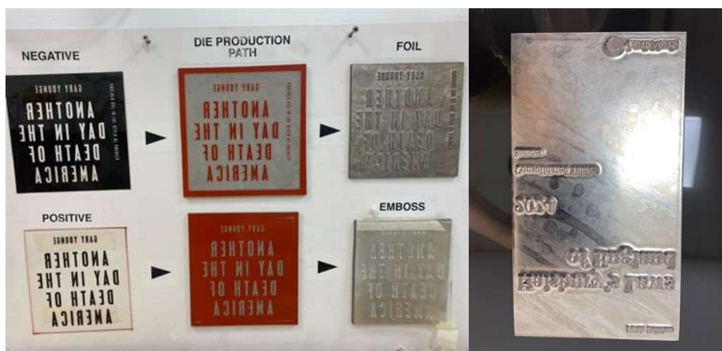
Figure 11a Evolution of foil artwork to create the brass-die. Figure 11b metal brass-die. Photo courtesy of Lisa Faratro, CPI
